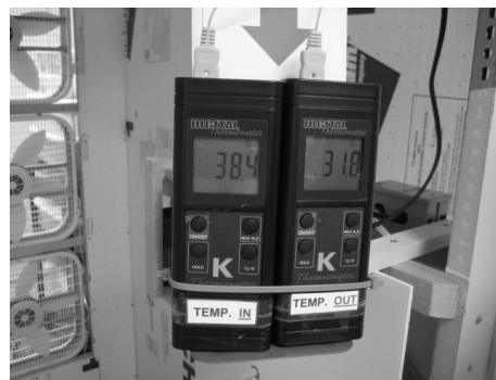
Figure 5: Temperature monitors showing manikin input air temperature and manikin output air temperature values which are needed to compute manikin heat loss values.
