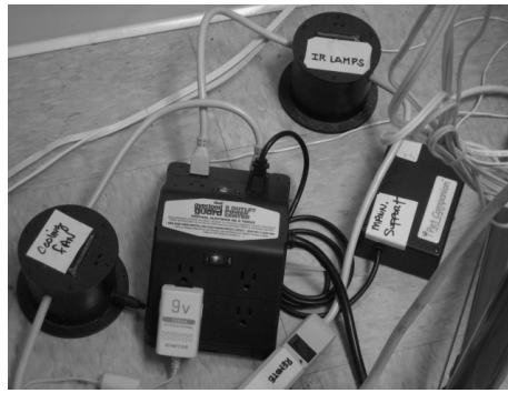
Figure 4: Remote control relays used in activating thermal manikin sub-systems.
